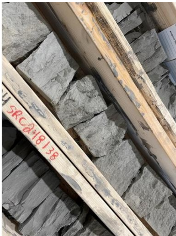
Figure 1. Core sample of the black shale deposit at the CEM warehouse in Saskatoon.
